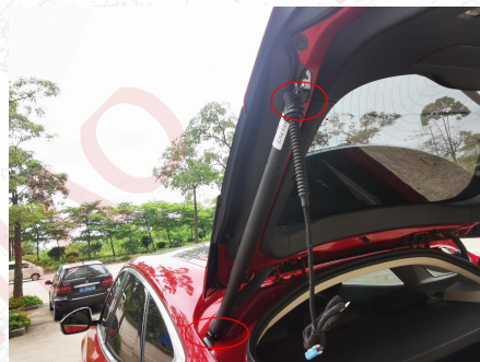
4、 Remove the original car gas spring, then install our electric struts.
