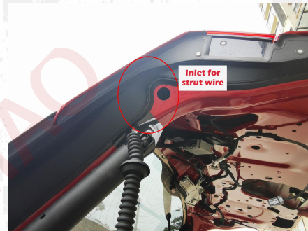
6、 Route the strut wire here.
