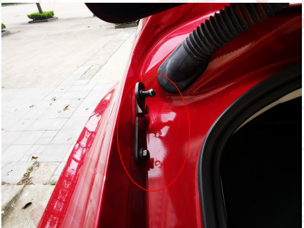
3、 Remove the original car brackets, then install our bracket.
