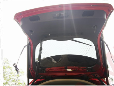
5、 Install our electric struts well (Note: the snap ring of the ball head cap must be in place, otherwise it will fall off the struts)
