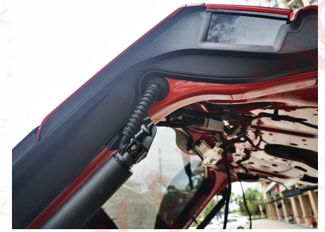
5、 Install our electric struts well (Note: the snap ring of the ball head cap must be in place, otherwise it will fall off the struts)
