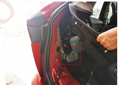
7、 Remove the original car lock, then install our lock hook. The lock driver is placed in the trim panel on the left side of the trunk.
