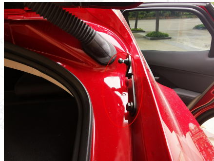
3、 Remove the original car brackets, then install our bracket.
