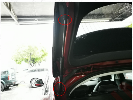
4、 Remove the original car gas spring, then install our electric struts.
