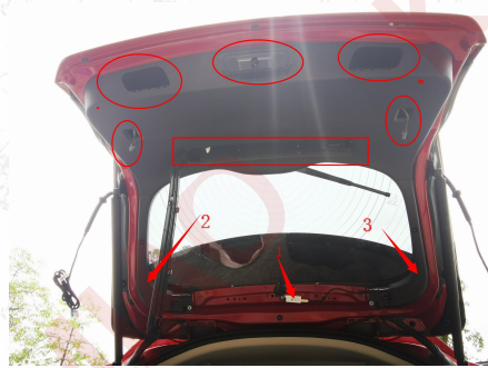
2、 Remove the trim panel and screws on the tailgate.
