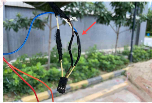
16. Unplug the original car lock signal plug, and connect the white wire on the right to our blue lock signal wire.
