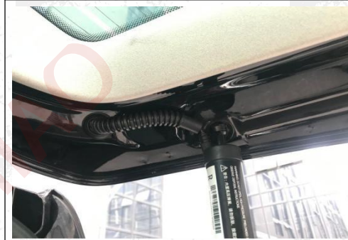
9. Punch a hole and route the strut wire on the right side.
