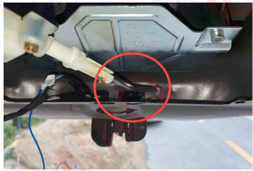
15. Unplug the 3 pin socket of the tailgate lock.
