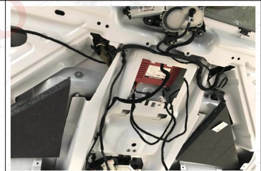
12. Connect and fix all the wiring harnesses of the control box as shown in the figure.
