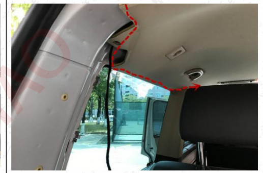
20. Remove the left decorative panel and thread the wiring harness to the main driver's seat.
