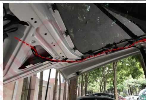
18. Route the power cord and signal wire to the front.
