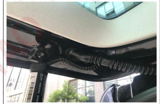
8. Punch a hole and route the strut wire on the left side.
