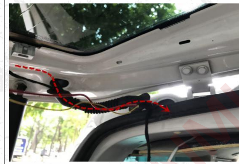
19. Route the power cord and central signal wire to the front along the red input wire.
