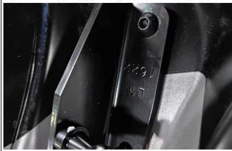
1. Install our bracket with original car screws. (Left and right side are the same)
