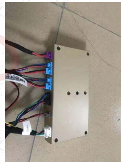
8. According to the plug color, insert the plugs into the control box (ECU)
