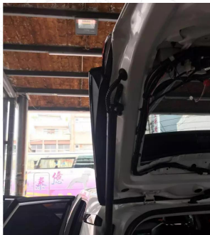
5. Install our electric struts.
