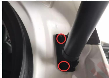
4. Remove the original car right lower bracket. Install our bracket and fix it with screws.
