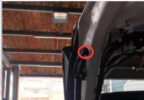
6. Drill a hole to route the strut wire and plug in the waterproof rubber.
