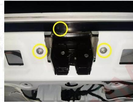
14. Remove screws in the yellow circle and the original door lock, install our top suction lock and fix it with the original car screw.
