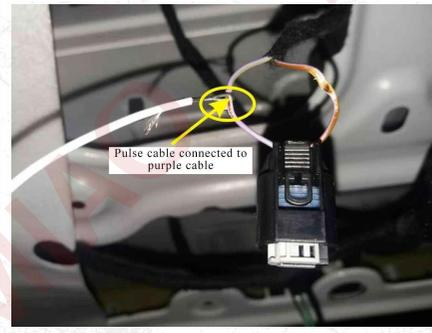
Pulse cable connected to purple cable
