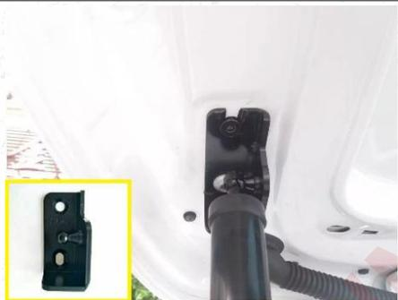
5.Install our upper left bracket (The ball head position is facing outward).and fix it with our screws.
