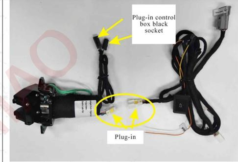
15. Insert our electric top suction lock socket as shown in the figure.
