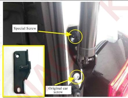
2.Install our lower right bracket.The top of the bracket is fixed with our screws and the bottom is fixed with the original car screws.
