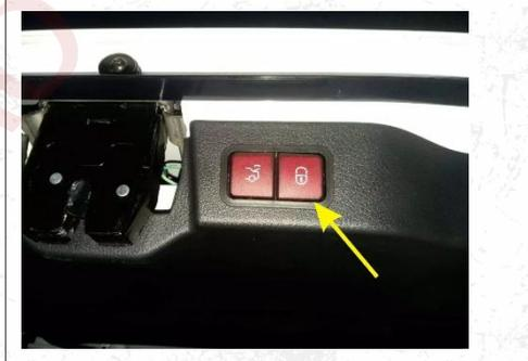
19. Cut a small square with the blade at the original tailgate trim panel and install our tailgate switch button.
