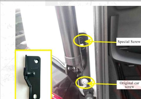
4.Install our lower left bracket.The top of the bracket is fixed with our screws, and the bottom is fixed with the original car screws.
