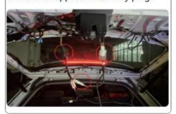
Ground wire location. Located inside the left side trim of the trunk
