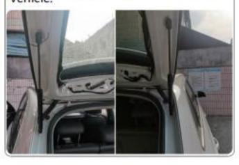
Remove the original car door ball head and install our matching ball head (same for left and right)
