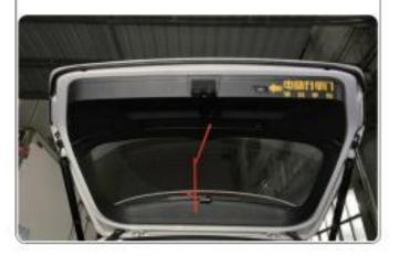
Remove the original car trim panel as indicated by the arrow in the figure below
