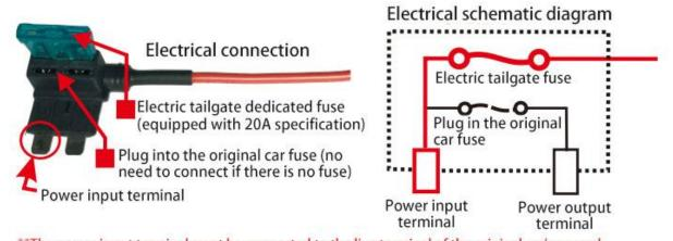
\*\*The power input terminal must be connected to the live terminal of the original car's normal power fuse hole. If connected in reverse, the original car's fuse will be blown due to overcurrent. Before installation, be sure to use a tester to measure and determine the power input terminal. The current flow is shown by the red line in the schematic diagram.
