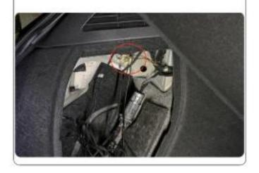
10. The location of the power supply is to find the fuse box under the main driving of the center console, and find the fuse in the position shown in the figure below. If you unplug the original car fuse, you must plug the fuse into our distribution power supply (Note: connect to 12V normal power and the fuse is above 20A)
