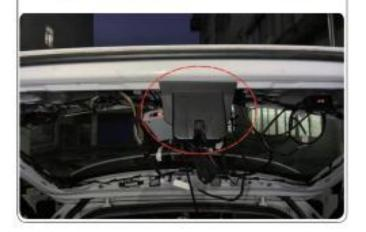
8.The lock block does not need to be connected to a plug. Unplug the original car lock block plug and plug it into the supplied three-way plug.
