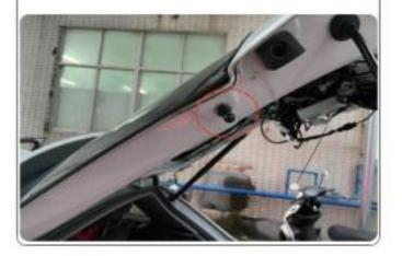
Schematic diagram of the electric strut installation (Note: After the strut is installed, please check whether the strut ball head card is in place and the strut line is facing the car door)
