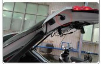
7. Install the self-priming lock block. Remove the original car lock block and install our self-priming lock machine.
