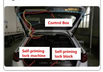
16. The hand buckle line is not connected
